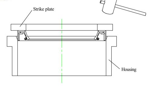
Simply pounding the seal into the housing can deform and permanently damage the seal
