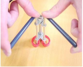
Keeping the u-cup in the kidney shape, insert the seal into position within the cylinder component and release the tool.
