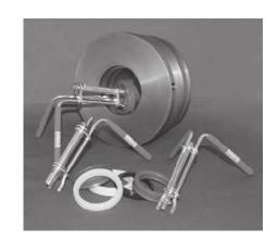
I hese tools aid U-seal installation, eliminating the risk of damaging the seal lip.
