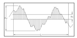
Ry (also Rmax) is the maximum roughness height in one cutoff length (L) of the profile.
