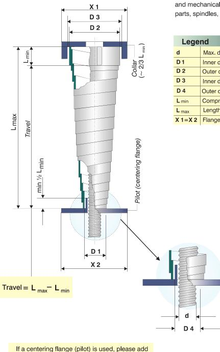
Safe protection against accidents, dirt, chips and mechanical damages on rotating machine parts, spindles, ball screws, shafts etc.
